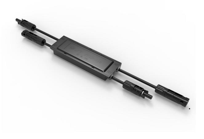
The XRSD-xyz meets SunSpec requirements,maintaining normal function by continually receiving a enable signal from the XTONG PLC Transmitter (PLC-2). The RSD executes rapid system shutdown when the Transmitter signal is absent. Users can manually execute rapid shutdown using Transmitter E-stop button.
